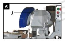
Use a wrench to unscrew a M20 X 40 hex head screw
