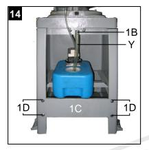
Attach the rear plate to the back of the stand.
