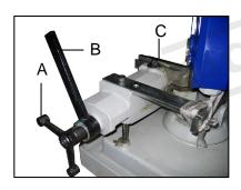
Use the hand wheel to open and close the vise jaw for work pieces that vary in width.
