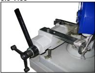
A clamping system that provides the basic support and security for the work material. Operations are conducted by hand-wheel, which opens and closes the vise jaws.
