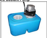
Found within the machine stand, the coolant pump is a self contained system that includes a tank, pump motor, filters and hoses.
