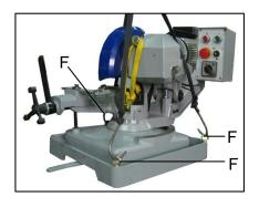
Prepare the machine unit for hoisting
